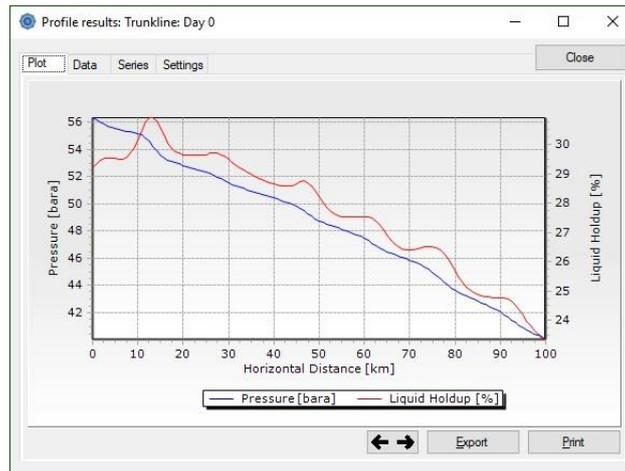
Figure 33: Trunkline profile with pressure and liquid holdup.
