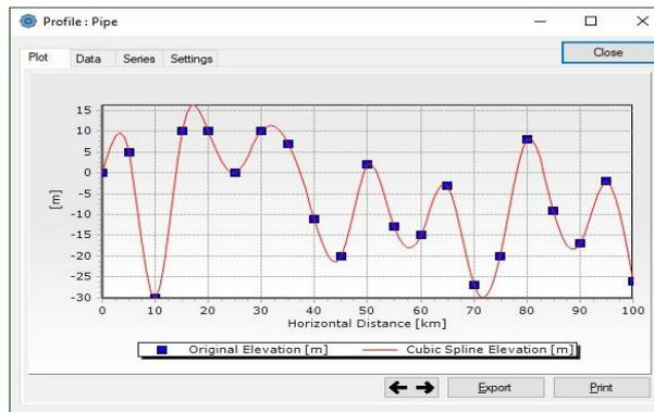
Figure 9: Trunkline elevation profile
