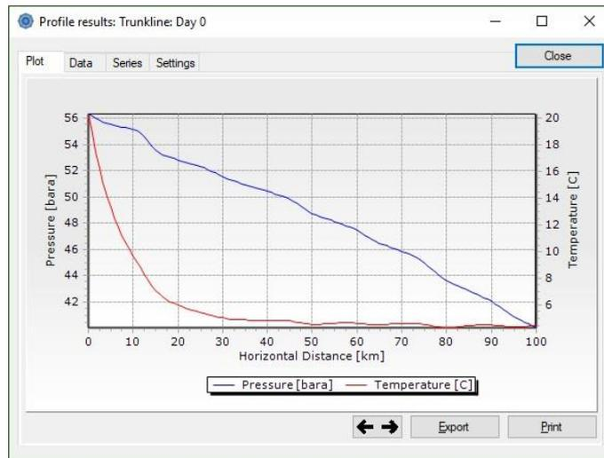
Figure 31: Trunkline temperature and pressure profile.
