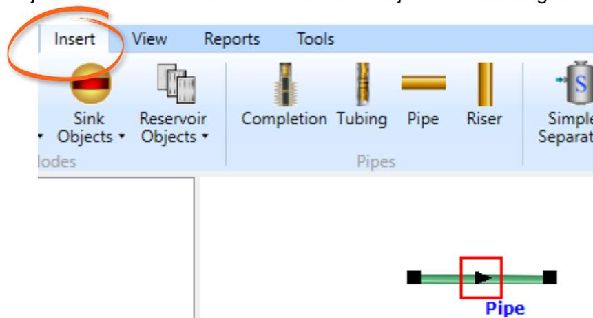
Figure 6: Adding a pipe object to the model canvas.
