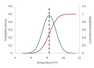
Figure 12. Uncertainty on temperature measurement
