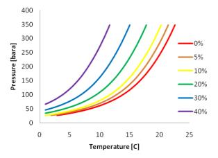
Figure 6. Hydrate dissociation curve for different MEG concentrations
