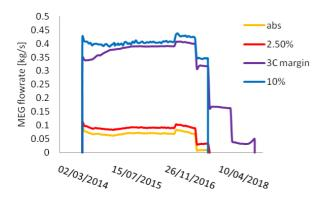
Figure 14. Comparison between MEG flowrates with different errors for the GNM-GFP flowline
